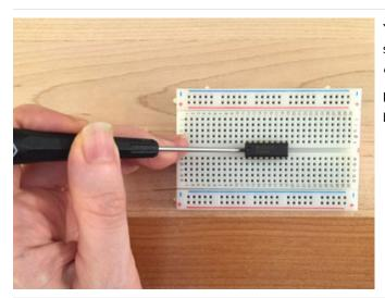
You can remove the chips easily by slipping a thin screwdriver or awl down the center ravine/divider and *carefully* prying upwards.
