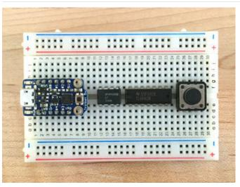
Then carefully press into the center of the breadboard. Watch out for bent pins!
