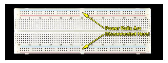
But some breadboards do not have the nice colored lines so you'll have to test with a multimeter or some other way to verify. Use little wires to jumper over the gap, if you want continuous conductivity
