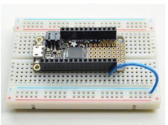
Plug in both ends into the breadboard as desired to make an electrical connection
