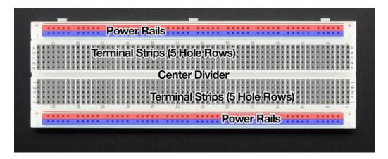
You put the components (buttons, LEDs, resistors, integrated circuits, etc) in the middle section, with each pin connected to the rows terminal strip. The power rails are long columns used to distribute the power and ground connections along the entire circuit.
