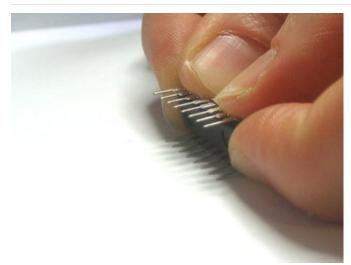
When new, the pins are not quite straight, they're bent out a little like an /--\ shape. You can carefully press the pins against a tabletop, and rock them forward together to bend into a |--| shape
