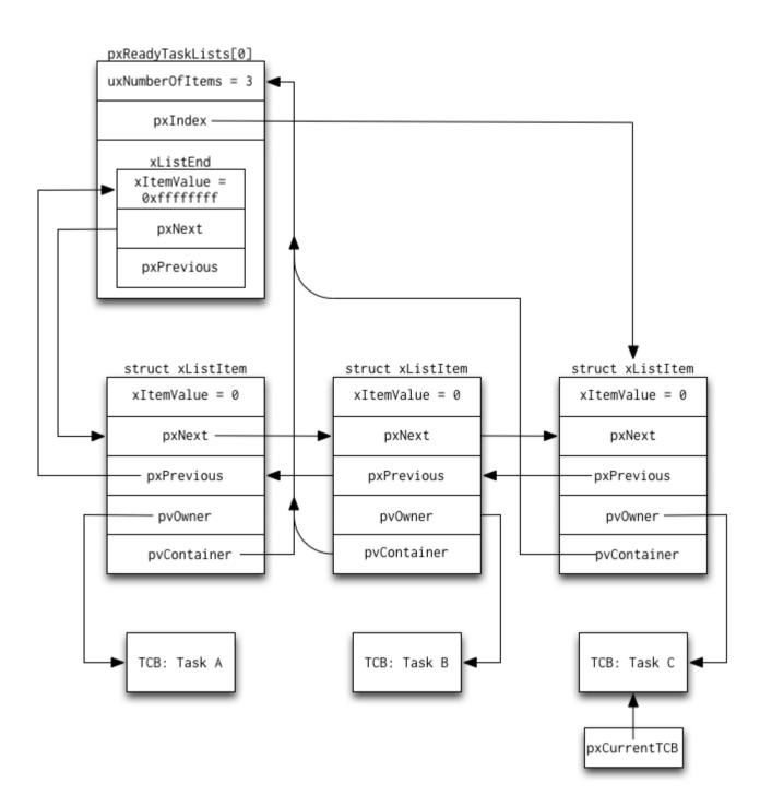
The pxReadyTasksLists[] list manipulation done in vTaskSwitchContext() is a good example of how pxIndex is used. Let's assume we have only one priority level, priority 0, and there are three tasks at that priority level. This is similar to the basic ready list picture we looked at earlier, but this time we'll include all of the data structures and fields.
