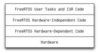
FreeRTOS ships with all the hardware-independent as well as hardware-dependent code you'll need to get a system up and running. It supports many compilers (CodeWarrior, GCC, IAR, etc.) as well as many processor architectures (ARM7, ARM Cortex-M3, various PICs, Silicon Labs 8051, x86, etc.). See the FreeRTOS website for a list of supported architectures and compilers.
